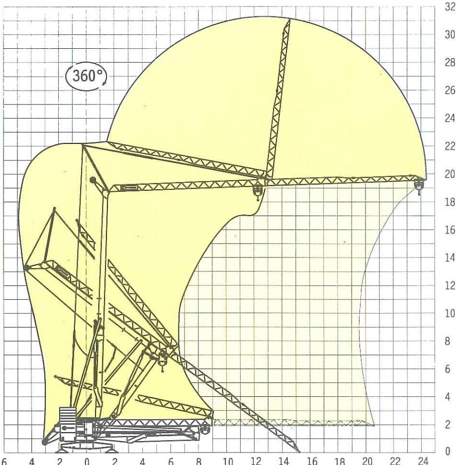
**Assembling:** Positioning and leveling on 360° - Assembling in few minutes in narrow places - Automated oleodynamic assembling with aerial opening of the jib - Remote-controlled independent movements of assembling - Safety valves on the whole system - Microswitch oil level in the gearbox
